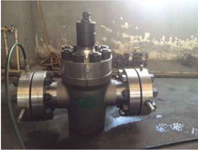
Pressure test for the gate valve
